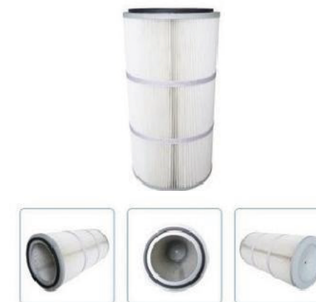
Model:G3566 Size:φ352*φ241*H660mm Filtration efficiency:100%(Particles≥5μm)
