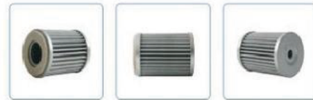
Model:G0.2 Size:φ50*φ28*55mm Filtering accuracy:10μm
