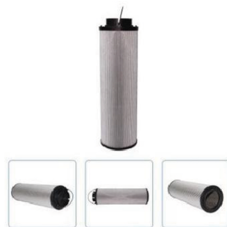
Model:1300R Size: \phi 143.5 \times \phi 96.5 \times 481.5 mm Filtering accuracy: 10\mu\text{m}
